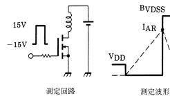
$R_G=25\Omega$   $V_{DD}=50V, L=1.74mH$
